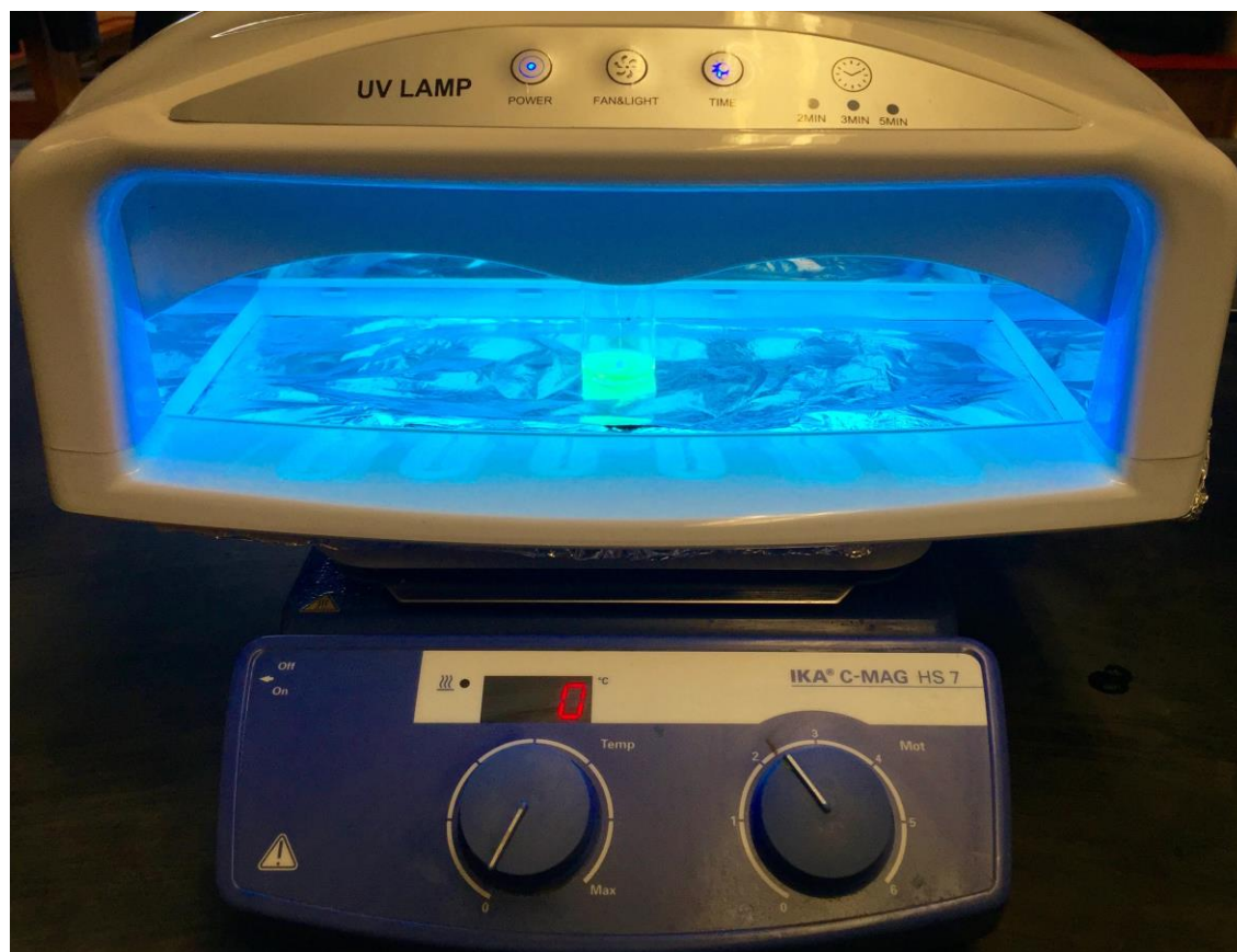
Figure S12. Photograph of the reaction setup for O-ATRP using UV irradiation.
