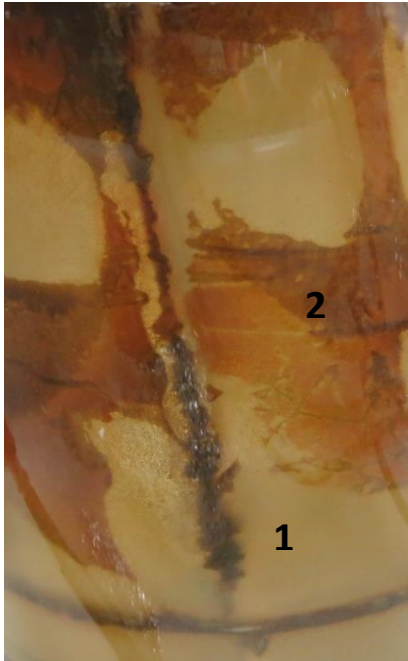
Figure S1 White (1) and brown (2) biofilm attached at the glass wall and metal surfaces in the continuous culture
