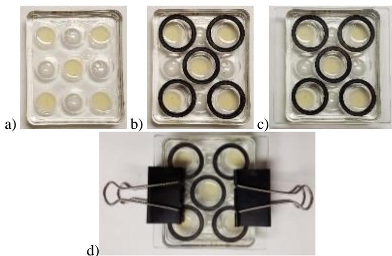
**Figure S1:** Step by step crystal growth apparatus set up.
