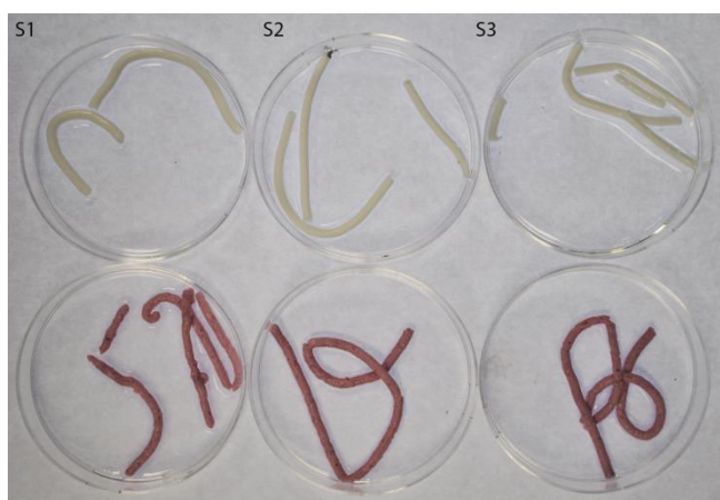
Figure S5. Cohesion test. Pictures from the CPC and the CPC/PFCE/gold pastes are shown after 24 hours incubation in PBS at 37 °C. On the top three samples from the CPC composite, while on the bottom the same amount of samples from the CPC/PFCE/gold composite. In the table are reported the score from the cohesion test. Score was attributed as follows: +++ = the paste broke in 1 single piece, ++ = the paste broke in > 2 pieces and <3 pieces, + = the paste broke in > 3 pieces.
