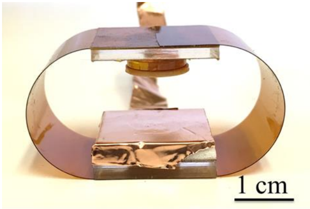
Supplementary Figure 8. Image of the TENG with the coupling of surface and dielectric polarization.
