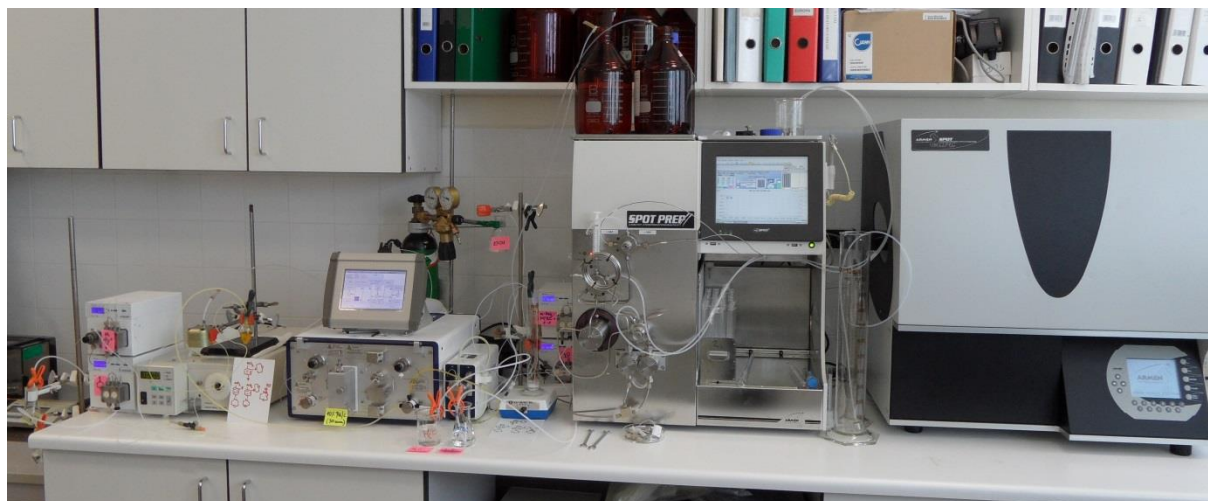
Figure S15. View of the coupled multistep continuous flow reaction with purification by MDM CPC with one-phase intake and asymmetric elution.
