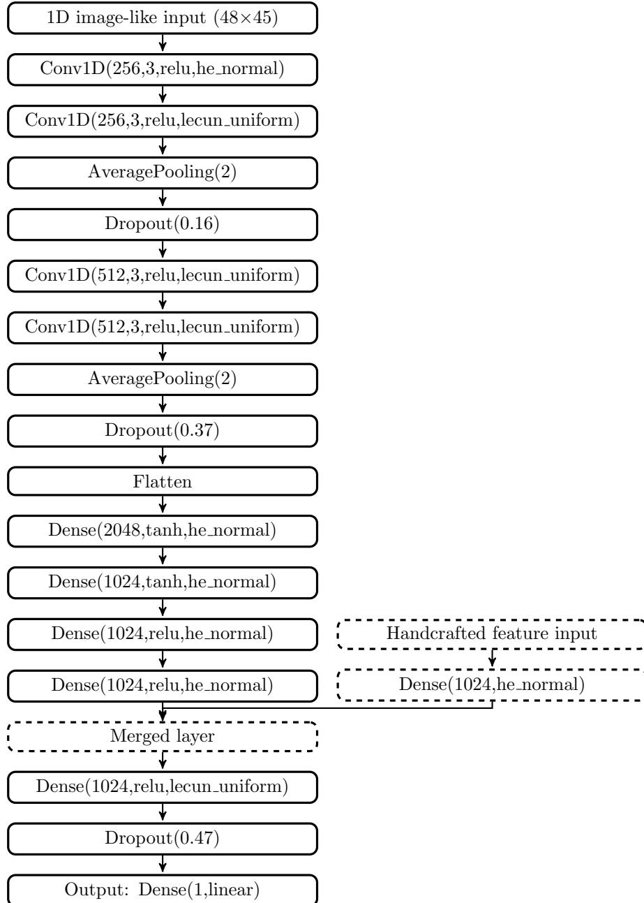
**Architectures of TNet-MMP-1 (single-task without the dashed part) and TNet-MMP-2 (multitask with the dashed part)**
