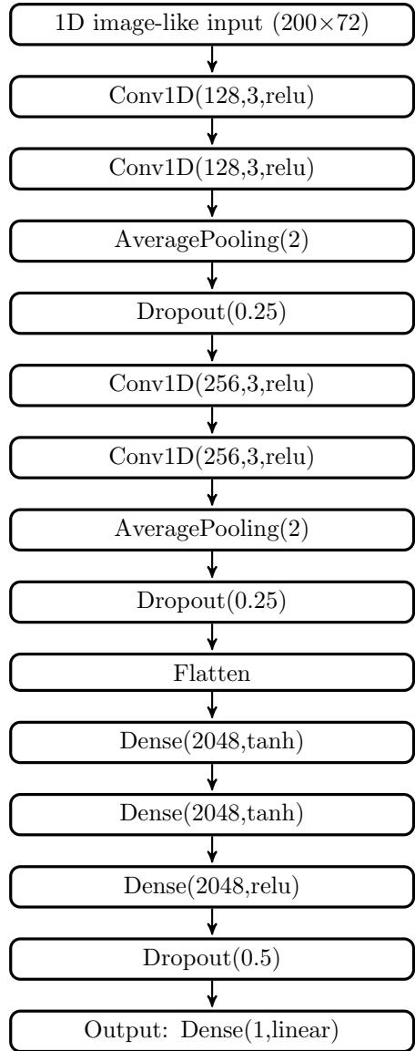
**Architectures of TNet-MP-1 (only topological input without the dashed part) and TNet-MP-2 (topological input and auxiliary features with the dashed part)**
