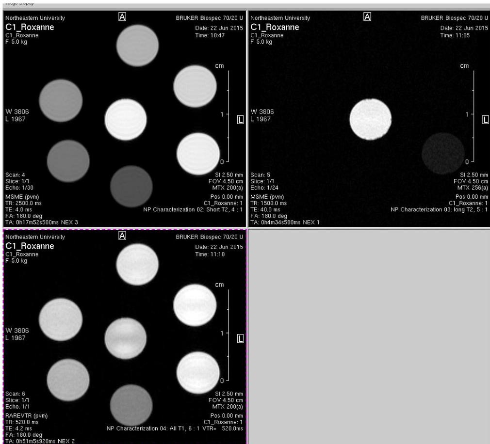
Supplementary Figure S9  $r_1$  and  $r_2$  maps of IONP-DHCA in solution that were generated at 7 T
