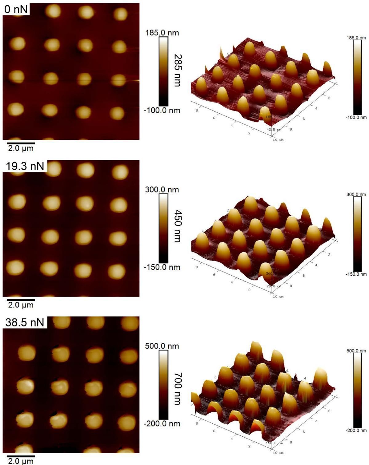
Figure S1: left: AFM height images of submerged pillar sample taken with different setpoints and corresponding 3D representation (right). Top: 0 nN, middle: 19.3 nN, bottom: 38.8 nN. Note the different height scales.
