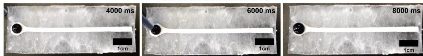
fig. S11. Response of the PVC side of the Janus bilayer to water. The wetting characterization of the opposing superhydrophobic PVC side of a 2 mm-wide strip of Janus bilayer on superhydrophobic nanofibrous substrates reveals no Mimosa Origami self-assembly.
