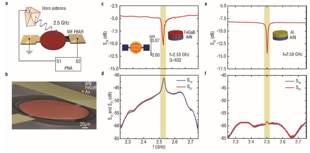
2. We simulated the electromechanical behavior of FBAR device. We show the simulated return loss curve ( $S_{22}$ ) and the out-of-plane displacement of the circular disk at its resonance frequency below. The detailed information can be found in the revised Figure 3 and the Supplementary section 7.
