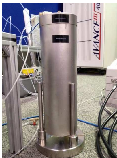
Figure S1: The automatic 'flow' mode polarizer used in this study.
