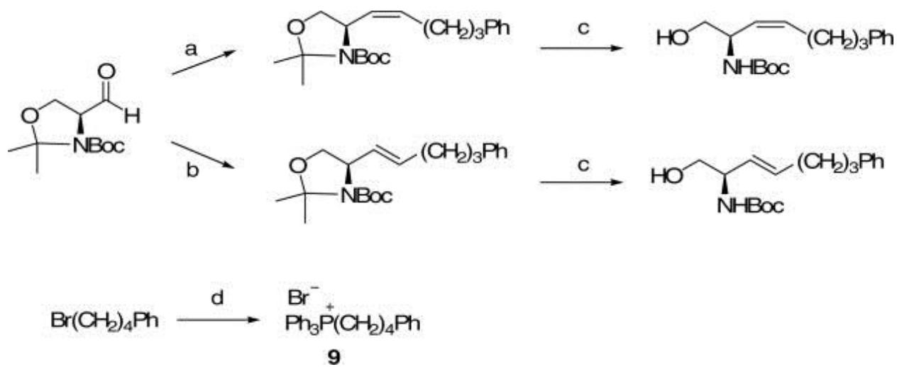
Supplementary Scheme 1. Reagents and conditions: (a) **9**, *n*-BuLi, THF, -78 °C–rt, 88%; (b) **9**, KHMDS, THF, MeOH, -78 °C–rt, 93%; (c) aq AcOH, rt, 94–95%; (d) PPh<sub>3</sub>, toluene, reflux, 99%.
