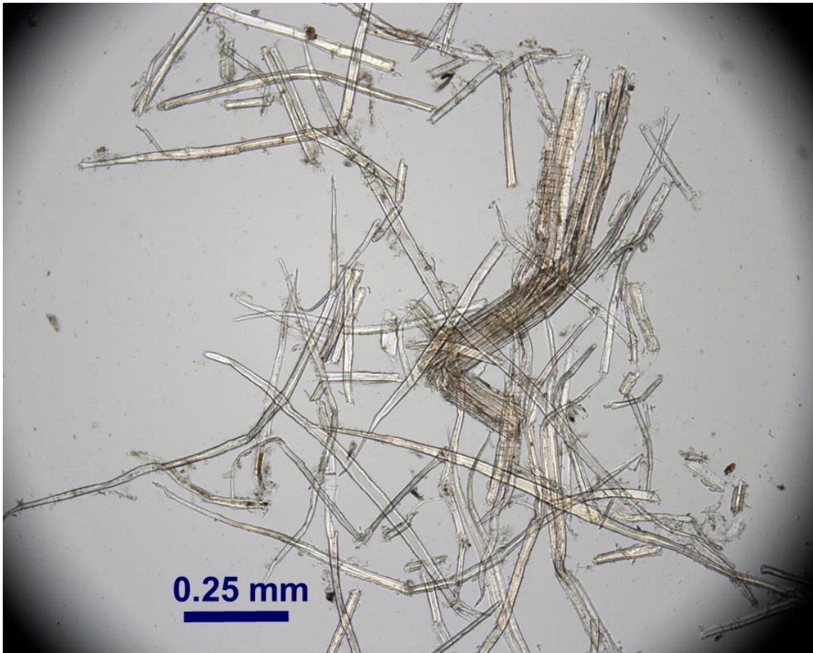
fig. S1. Optical microscopy images of wood fibers produced using p -TsOH fractionation under low-severity conditions (fiber lignin content, 16%), followed by mechanical refining to 550-ml Canadian Standard Freeness.
