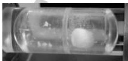
Fig S6.1: Powder "snow-balling" within the milling jar at 20 Hz.
