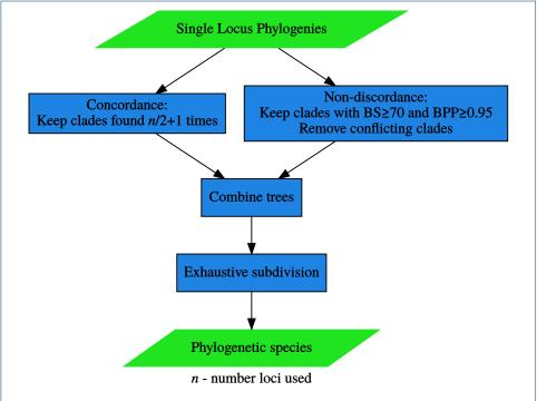
**Figure S3 Flowchart of the GCPSR method** *sensu* **Dettman** *et al.*. Green parallelograms are input and output files. Blue boxes are the scripts, roman numerals indicate the algorithmic steps. BS - bootstrap support value, BPP - Bayesian posterior probability value.
