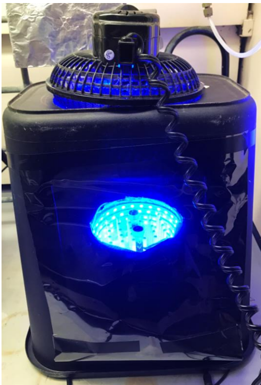
Figure S7: Procedure B photoredox cross-coupling reaction set-up (0.50 mmol scale)
