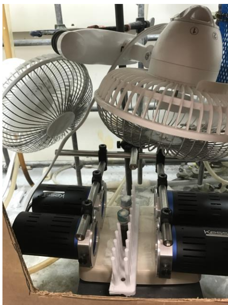
Fig S8: Procedure A and C Kessil lamp setup for shortened reaction times (0.25 – 0.50 mmol scale)
