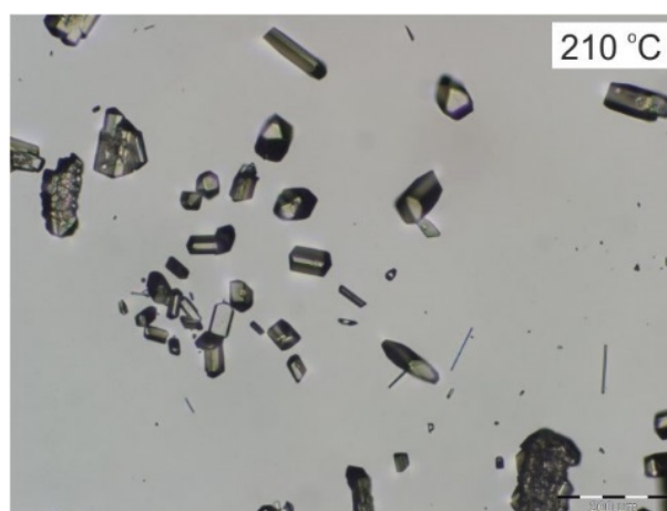
Figure S9. Morphine sublimates. Note that all of the crystals correspond to the same polymorphic form, M-I°.
