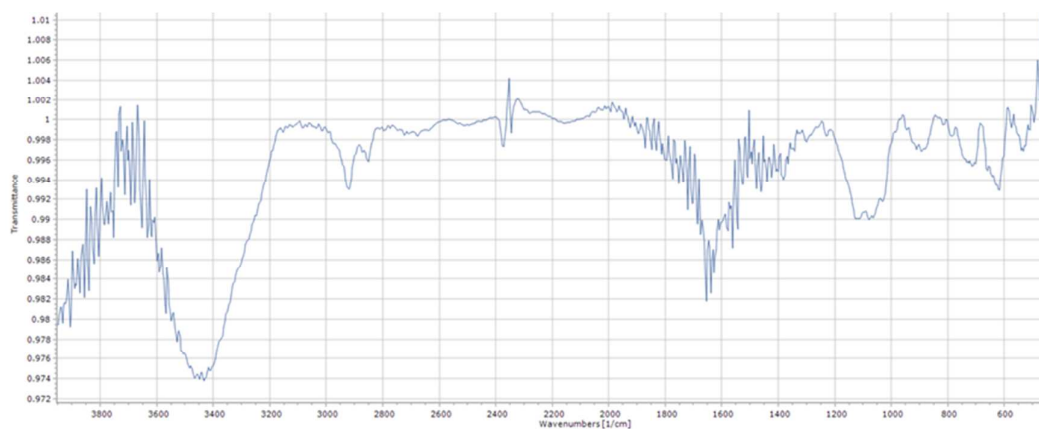
Figure S14. IR spectrum of Lewis X/tetramannoside AuNPs. IR (KBr): \nu = \sim 3600–3100 (br), 2906, 2845, 1638, 1094.
