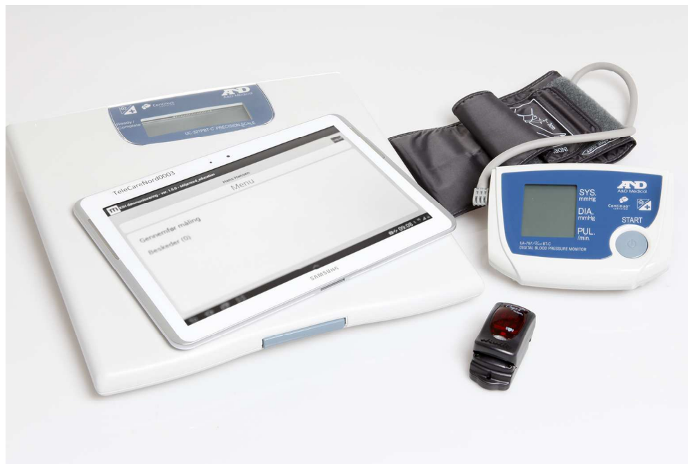
Figure 1: The Telekit system consists of a tablet, a blood pressure monitor, a fingertip pulse oximeter and a health precision scale.
