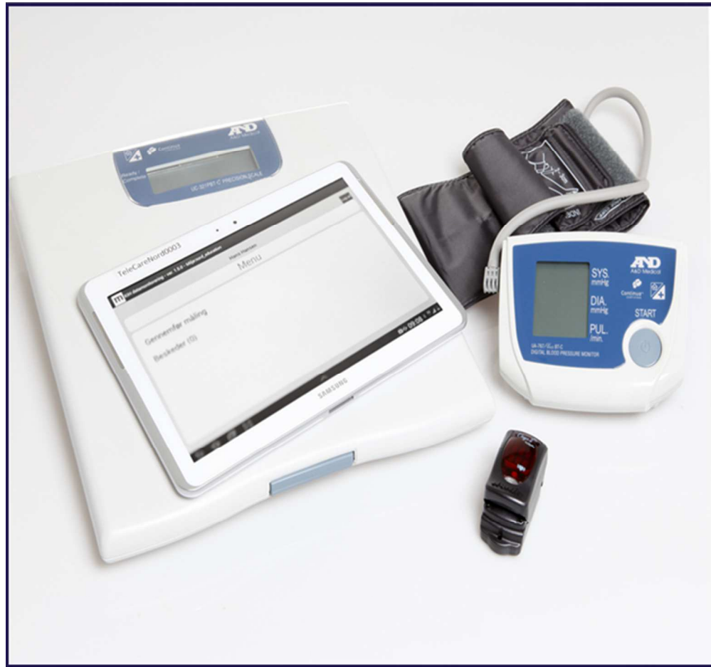
Figure 1: The Telekit system consists of a tablet, a blood pressure monitor, a fingertip pulse oximeter and a health precision scale.
