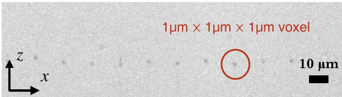
Figure S4: IR microscope image from single-pulse modified volume. The x - z cross-section is imaged with IR microscopy. Voxels of \approx 1\text{-}\mu\text{m} feature size are created with \approx 8\mu\text{J} laser pulses. The laser propagates along the z axis as in the manuscript conention.
