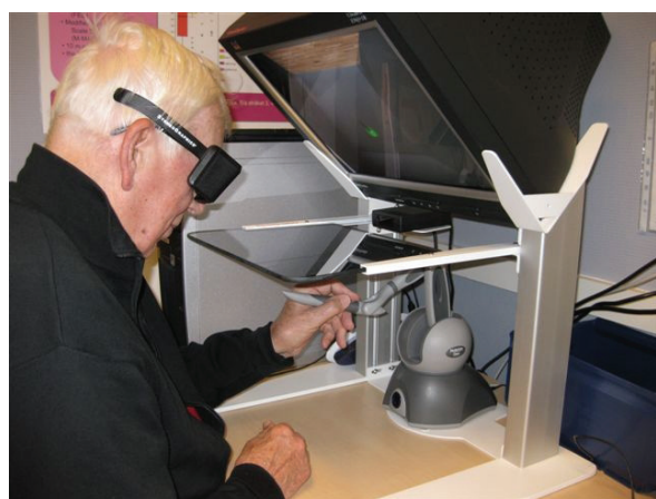
Figure 3 Participant is performing the VR-test. The VR equipment consists of a semi-immersive workbench with haptic device and stereoscopic glasses.
