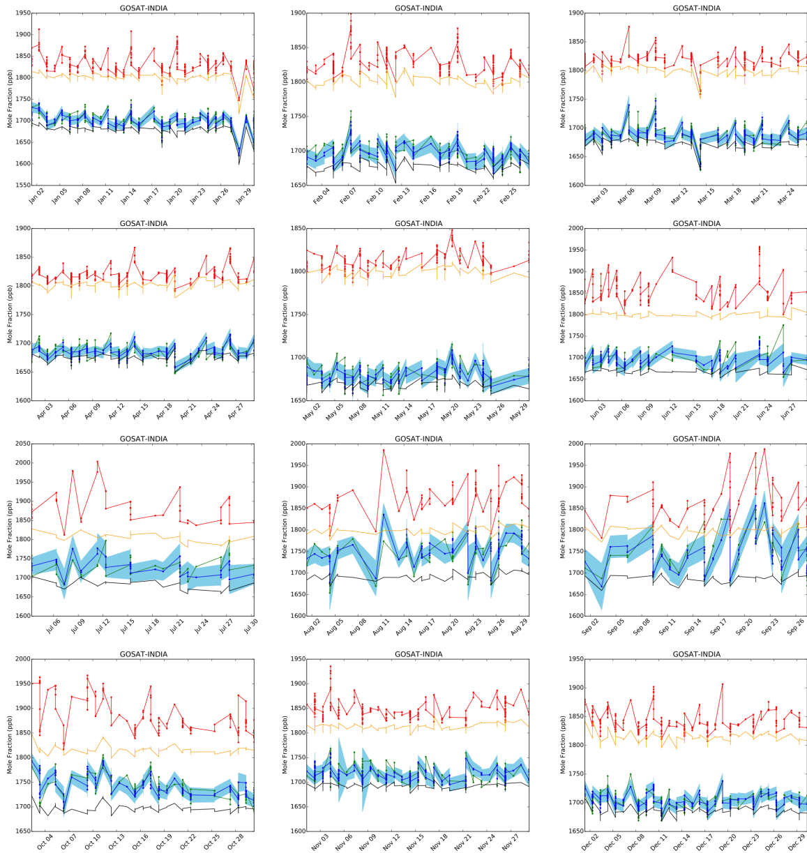
Supplementary Figure 16: GOSAT observation and model comparison (ppb) for 2013. Prior (red) and posterior (blue) mole fractions and prior (orange) and posterior (black) boundary conditions. Observations are shown in green with blue shading indicating the 5-95 th percentile range of the model-measurement error derived in the inversion. Mole fractions represent the term XCH_{4,pert}^{model} in equation (6).
