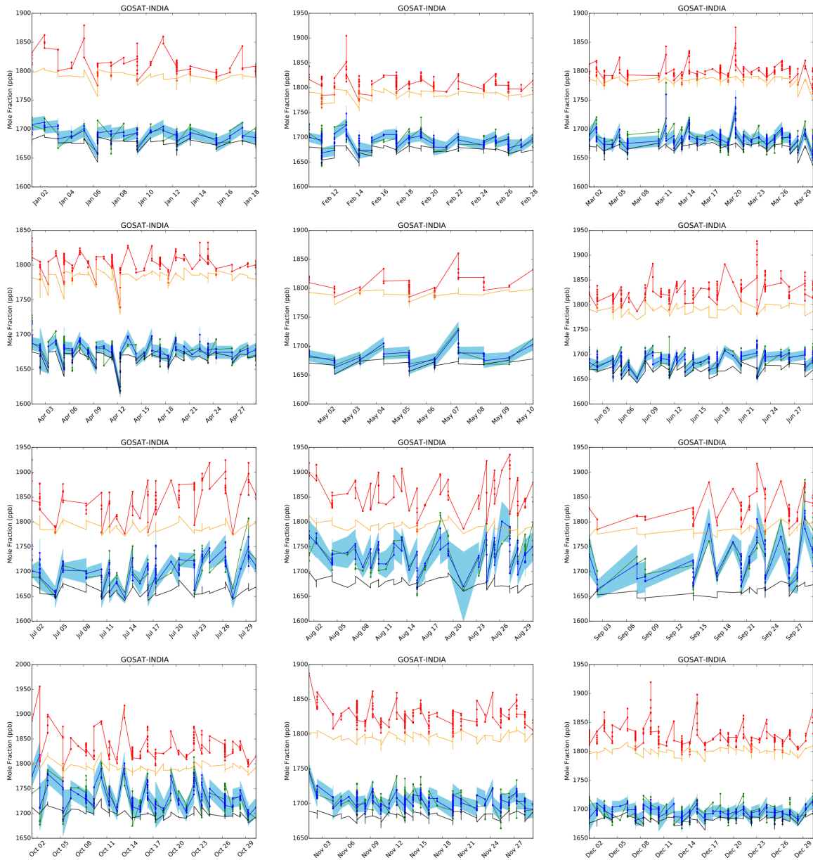
Supplementary Figure 15: GOSAT observation and model comparison (ppb) for 2012. Prior (red) and posterior (blue) mole fractions and prior (orange) and posterior (black) boundary conditions. Observations are shown in green with blue shading indicating the 5-95 th percentile range of the model-measurement error derived in the inversion. Mole fractions represent the term XCH_{4,pert}^{model} in equation (6).
