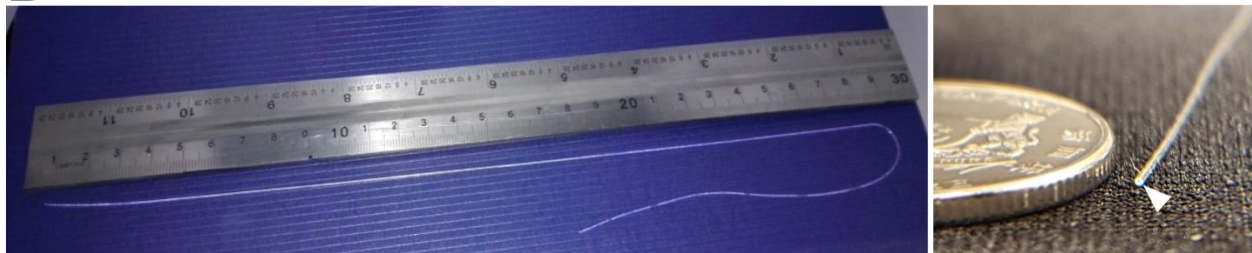
Fig. S2. Photos of (A) PDMS microtubes with different inner diameters (ID) and (B) left, a 45 cm long PDMS microtube with ID = 50 \mu\text{m} and right, the opening of the microtube (white arrow).
