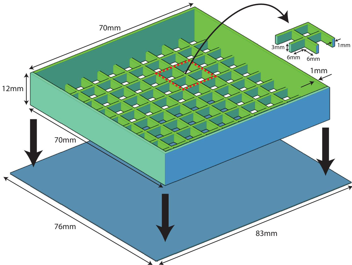
Supplementary Figure 1. Design of imaging chambers for 3D printing.
