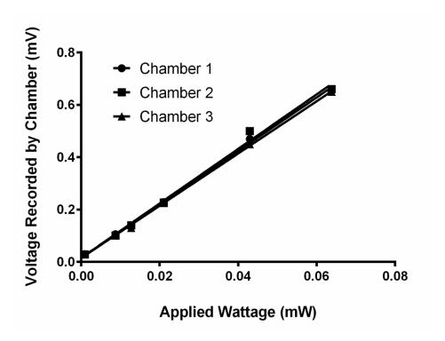
Supplementary Methods Figure 1 Calibration curve of purpose built calorimeter.
