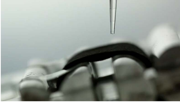
Movie S1. An 8- \mu L water droplet moving fluently down off the inclined superhydrophobic surface at strain = 0%.
