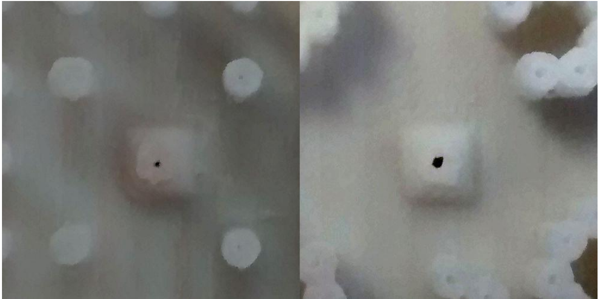
Supplementary Figure 3. Device outlet holes differences. Although both devices were printed under the same conditions, differences can be seen in the size of the outlet hole.
