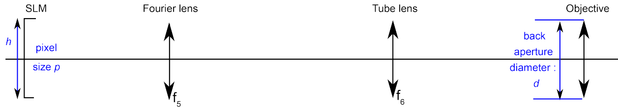
Supplementary Figure 4: Simplified diagram of the optical system (hologram synthesis section). We define the effective area of the SLM, h , and the pixel size, p . The Fourier lens, tube lens, and objective, and their respective focal lengths, and d , the back-aperture diameter of the objective.
