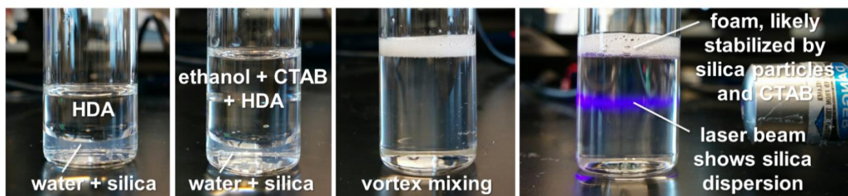
Supplementary Figure 12: Mixing of water, HDA and ethanol (with silica nanoparticles and CTAB as additives).
