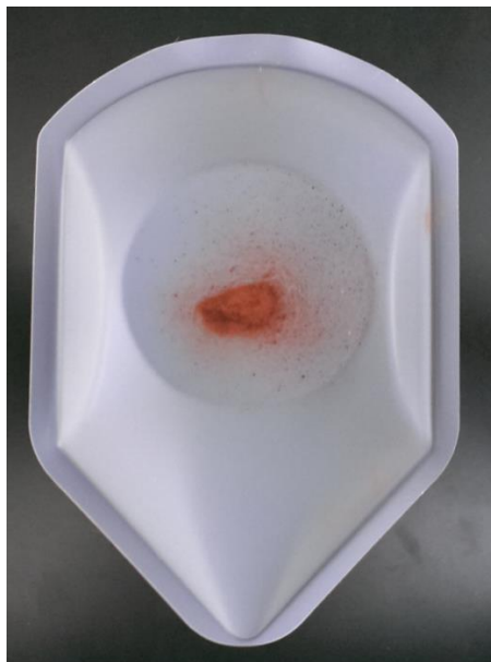
Supplementary Figure 31: Photograph of the 50-Mg 50-Fe 3+ precipitate (150° C) after drying in-vacuo and grinding to a fine powder in a mortar and pestle.
