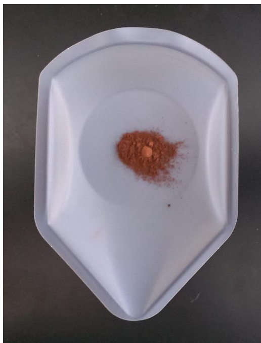
Supplementary Figure 19: Photograph of the 100\text{-Fe}^{3+} precipitate ( 100^\circ\text{C} ) after drying in-vacuo and grinding to a fine powder in a mortar and pestle. Note the reddish color which is likely from the presence of \text{Fe}^{3+} .
