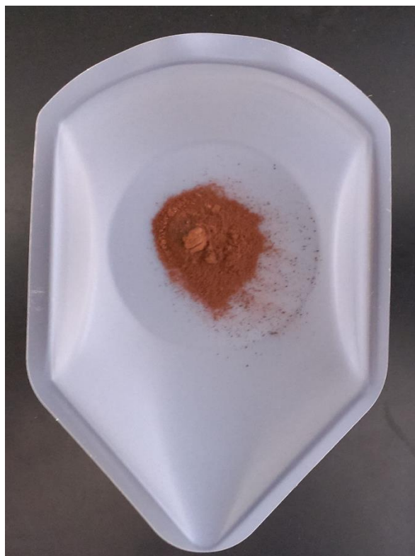
Supplementary Figure 27: Photograph of the 15-Mg ^{85}\text{Fe}^{3+} precipitate ( 100^\circ\text{C} ) after drying in-vacuo and grinding to a fine powder in a mortar and pestle.
