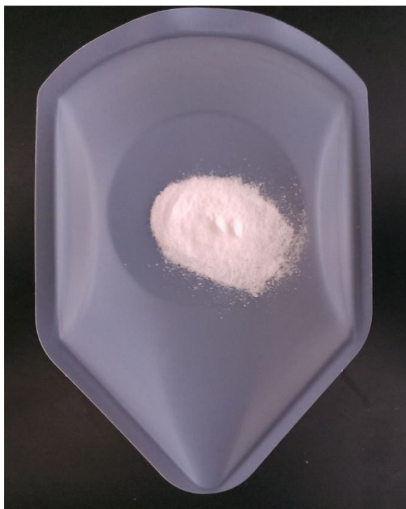
Supplementary Figure 23: Photograph of the 100-Mg precipitate aged at 100° C after drying in-vacuo and grinding to a fine powder in a mortar and pestle.
