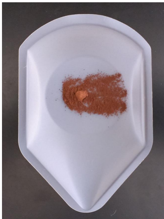
Supplementary Figure 36: Photograph of the 10-Mg 90-Fe 3+ precipitate at 150° C, after drying in-vacuo and grinding to a fine powder in a mortar and pestle.
