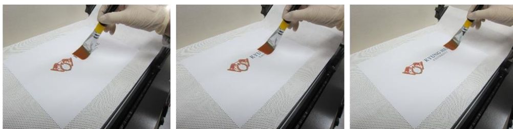
Figure S2. (a) Heated mount for brush painting and (b) brush painting process of Ag NW/PEDOT:PSS film on PU substrate using a typical flat paintbrush.
