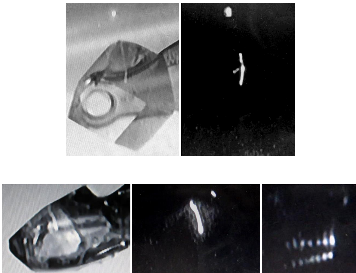
Figure S4 The flux density in the unattenuated beam generated optically visible fluorescence in the X-ray illuminated region at all temperatures. (Top) A lysozyme crystal at 260 K, with the beam hutch lights on (left) and off (right), as viewed through the beamline telescope. (Bottom) A lysozyme crystal at 100 K. The right-hand frame shows the fluorescence afterglow following six consecutive exposures separated by 1 s. At 260 K the fluorescence faded immediately, but at 100 K it persisted for ~6-8 seconds. Shape and brightness variations of the cylindrical illuminated crystal regions are due to reflection and refraction from crystal facets.
