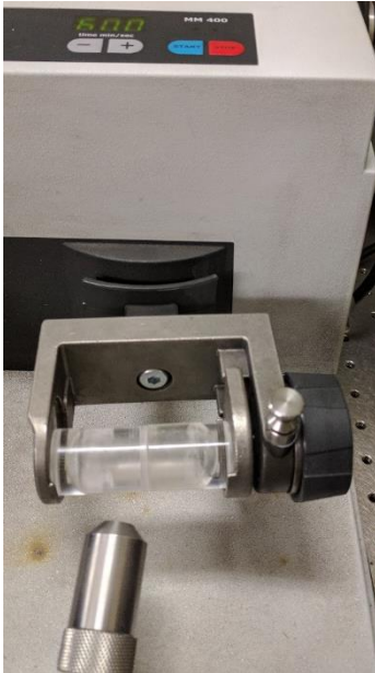
Figure S2: Picture of the experimental setup, showing a 15 mL volume PMMA jar mounted on a milling station of the Retsch MM400 mixer mill and the tip of the Raman spectroscopy probe.
