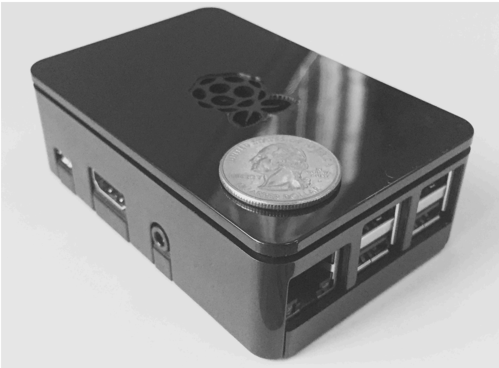
Figure S5. Raspberry Pi microcomputer used to continuously acquire and transmit ventilator waveform data over the health system wireless network to a study server. Raspberry Pis are connected to a serial port on the back side of the ventilator user interface screen using an RS232-to-USB null modem and secured out of sight.
