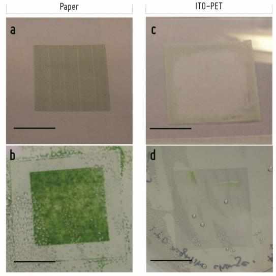
Comparison of the growth of printed *Synechocystis* cells on copy paper (a, b) and ITO-PET (c, d). Panels a and c show freshly printed cells and panels b and d the growth after 7 days of incubation on solid medium (BG-11, agar 1.5 % w/w). Each scale bar measures 1 cm.
