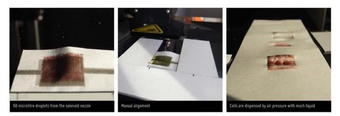
Inkjet printing of cyanobacteria using a research-grade microvalve-based cell printer. The cyanobacterium *Thermosynechococcus elongatus* BP-1 and redpigmented cyanobacterium *Phormidium persicinum* PML 715 were printed using a Celljet (Cronus Technologies, UK). The pattern was programmed in the custom software to a basic 20 x 20 mm square. The far-left panel shows a
