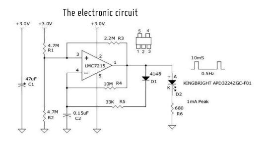
LED circuit. Photograph of the circuit (upper panel) and the electronic circuit diagram (lower panel).
