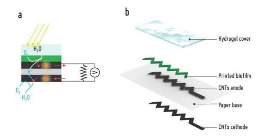
'Sandwich' design for the fully printed BPV device. Schematic representation of another system for the printed paper-based BPV cell in which the anode and cathode are back to back with the paper substrate in between (a). Expanded construct of the sandwich structure (b).
