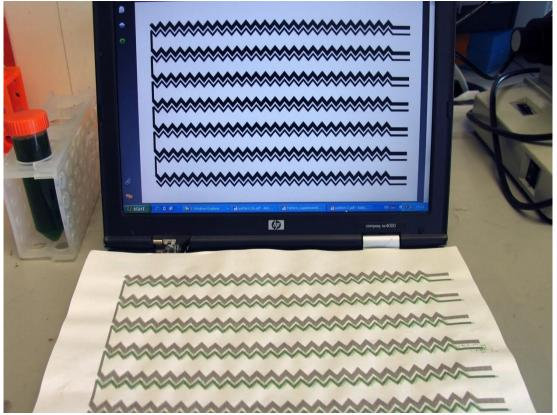
Printing of an A4-size fully printed BPV cell for bioenergy wall paper. The panel shows a freshly printed A4-size BPV 'paper' containing zigzag electrodes in series, shown together with the computer-aided design file on the computer screen. Green zigzag lines are anodes of printed *Synechocystis* cells on top of preprinted CNTs.
