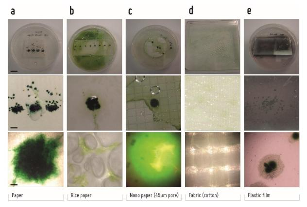
Testing biofilm growth of printed *Synechocystis* on various materials. Photographic comparison of the growth of inkjet-printed *Synechocystis* (WT-G) on various inkjet-printable sheet substrates following 14 days of incubation: Copy paper (a), rice paper (b), nano paper (c), cotton fabric (d), and inkjet plastic film (e). There are three scale bars, one per row: from top, each measures 1 cm, 1 mm, and 100  $\mu$ m respectively.
