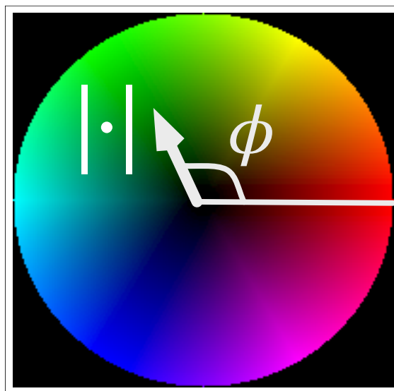
Fig H. Hue-Brightness Model For Rendering A Pixel From Complex Datum. To represent a complex-valued datum as a pixel in an image, distance from the origin in the complex plane ( |\cdot| ) is rendered as brightness and phase ( \phi ) as hue. In this paper, the rendering model may be represented mnemonically in figures by the icon on the right.
