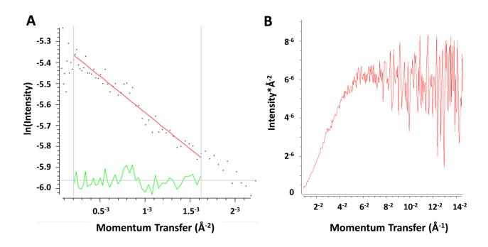
Figure S4. Analysis of MAL 123-218 SAXS data. (A) The Guinier plot of the low scattering angle (Å<sup>-2</sup>) region of the SAXS data fits well to a linear regression (red line) with low residuals (green line), indicating that the RNA was not aggregated. (B) The Kratky plot shows a leveling off as momentum transfer/scattering angle increases, indicating that the RNA is non-globular, but well-folded and extended in solution.
