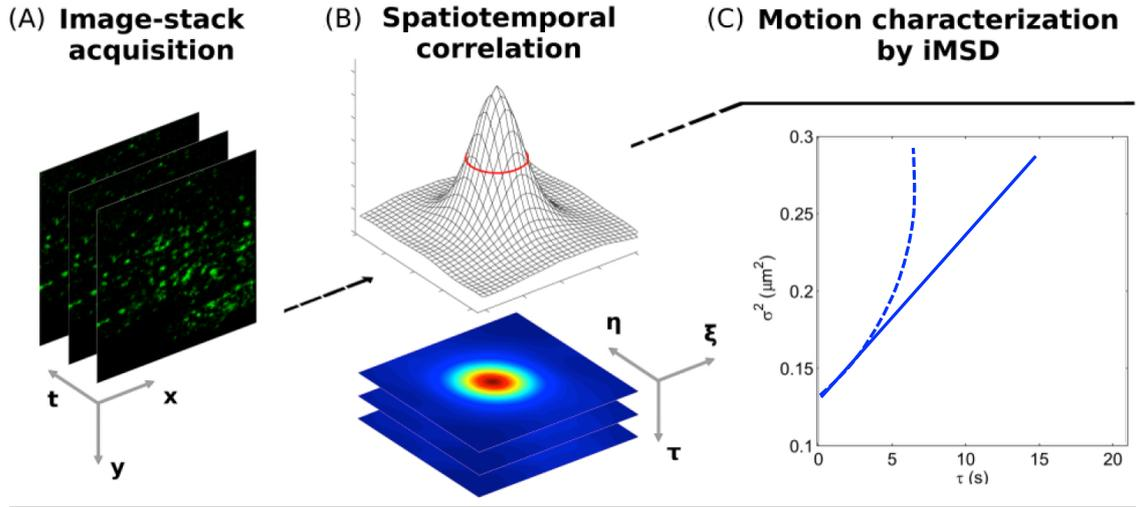
**Figure S1.** (A) Sequential image series are collected by a confocal microscope. (B) The spatiotemporal correlation function  $g$  of the fluorescence fluctuations  $\delta i$ , which are recorded pixel by pixel and frame by frame is calculated by the following relation:
