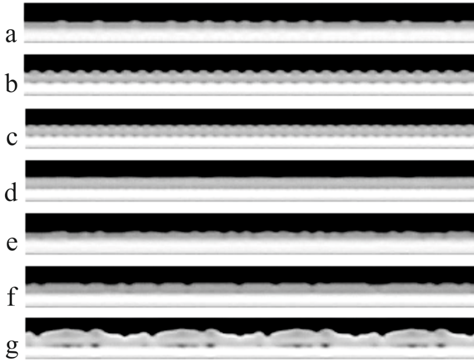
Supplementary Figure 10 | Plasma density contours at 240 ns from the current start. (a): initial perturbation seed is produced by the real thermo-elasto-plastic dynamics of the material (our study), (b, c, d): the seed is generated by an artificial sinusoidal function with 1.5 larger (b), equal (c) and 1.5 smaller (d) wavelength but same amplitude as in (a), are used respectively as initial seed. (e, f, g): random seed perturbation functions (e, f) and a multispectrum periodic function (g) are used as initial seed respectively.
