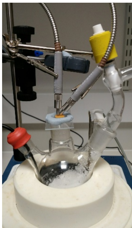
Supplementary Figure 4 Photograph of the setup used to determine the sensitivity of the films of complex 1 coated on glass to atmospheric water vapour. In a sealed three-neck round-bottom flask, a film of 1 , initially in the anhydrous Form-II phase, is held under nitrogen gas at atmospheric pressure (central neck). The flask contains a LiCl(sq) slurry and is kept in a Polar Bear Plus reactor to allow the water vapour concentration to be controlled (bottom). A thermocouple is inserted through a rubber seal to allow the temperature of the solution to be monitored (left neck). A light source and reflectance probe are positioned at 45 ° to record reflectance spectra through the supporting glass slide (top).
