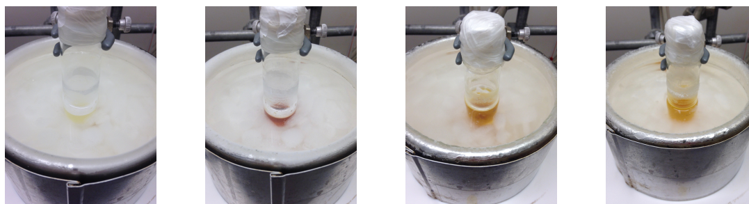
10 min after addition of Et 2 B-OTf 30 min after addition of DIPEA 10 min after addition of aldehyde 2h after addition of aldehyde
