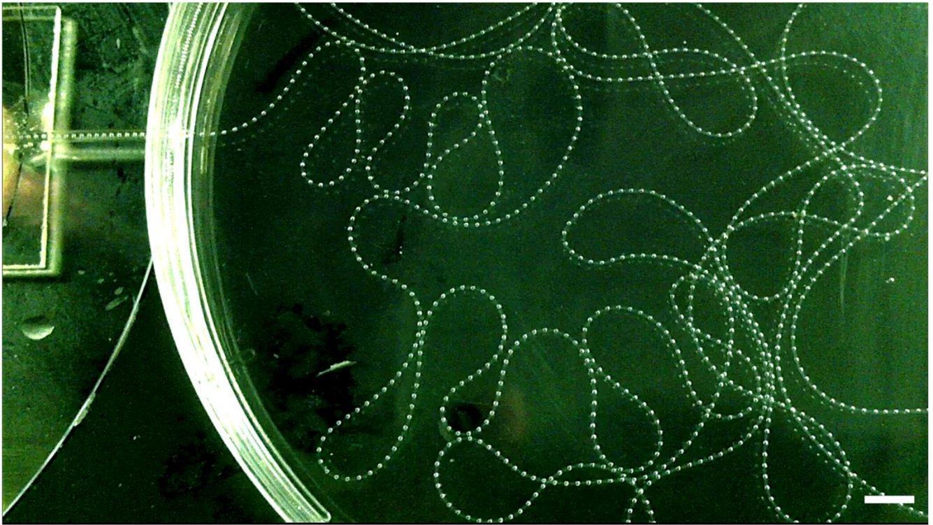
Supplementary Figure 1 | The optical image showing the fabrication of the cavity-microfiber. The ABC solution wrapping gas bubbles was extruded from the orifice into \text{CaCl}_2 solution and ABC solution can be crosslinked instantly into gelatinized alginate calcium fiber upon touching with the \text{Ca}^{2+} ions. Scale bar, 4 mm.
