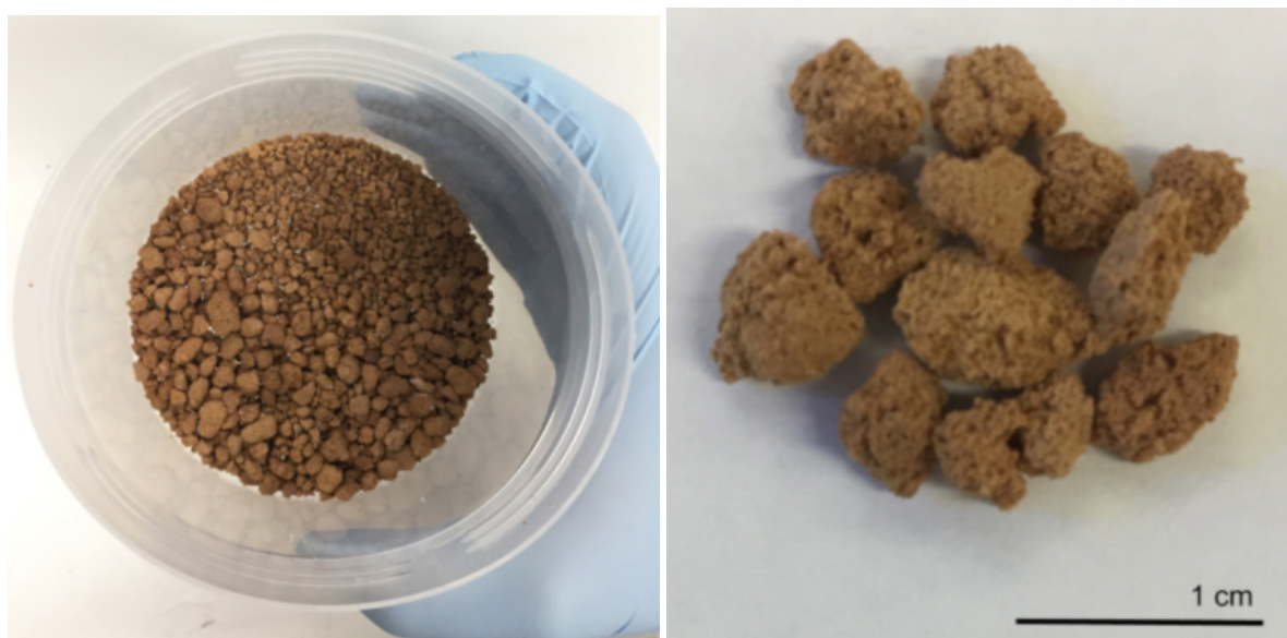
Fig. S57 | Samples of the porous canola oil polysulfide (50% sulfur) prepared using sodium chloride as a porogen.
