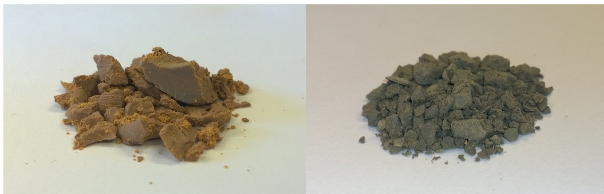
Fig. S35 | Canola oil polysulfide before and after treatment with mercury chloride Left: Canola Oil Polysulfide synthesised before treatment with mercury chloride Right: Canola Oil Polysulfide synthesised after treatment with mercury chloride (20 mg/mL, 24 hours). The material changed colour (from brown to grey) after binding the mercury.
