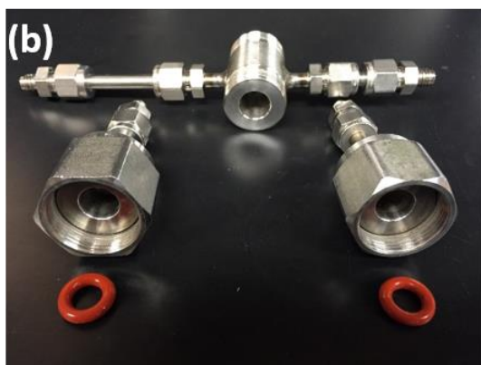
Supplementary Figure 7. (a) Schematic diagram of gas permeation system. (b) and (c) Photographs of hollow fiber permeation cell.
