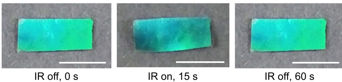
Figure S4. Photographs (top view) of reversible twisting and untwisting of the laminated film in response to global IR irradiation. The top-view photographs are taken at the fixed angle that is perpendicular to the substrate. Scale bar: 5 mm.
