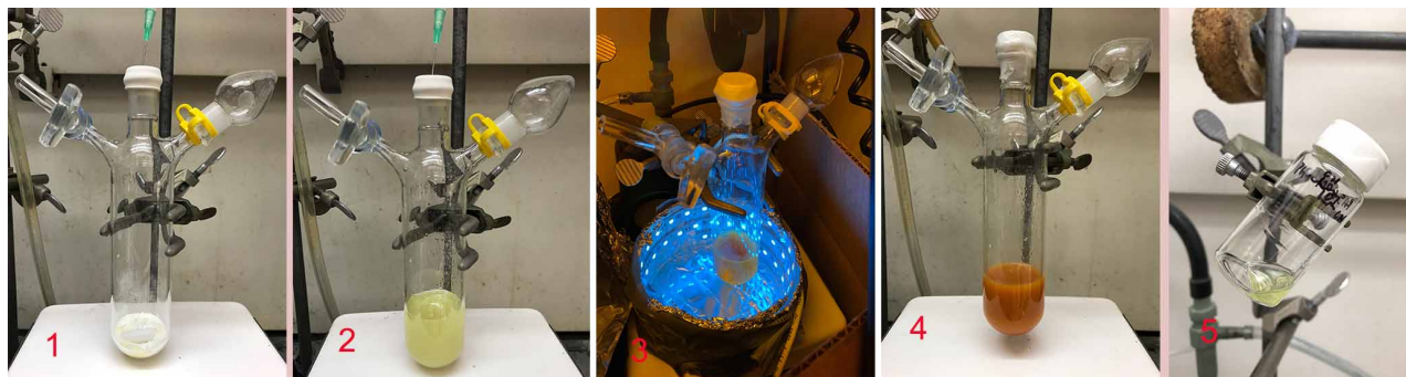
Figure A: 1. Reaction components were added to a Schlenk tube and then purged/evacuated with N_2 . 2. Reaction mixture in dioxane. 3. Schlenk tube was placed in blue LED chamber while a fan was placed at the top to keep the temperature nearly at 25\text{ }^\circ\text{C} . 4. Reaction mixture after 24 h. 5. Isolated compound.
