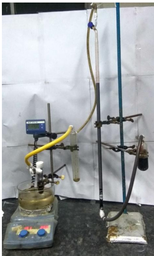
Supplementary Figure 118. Setup for hydrogen gas evolution (a volumetric quantitative analysis).
