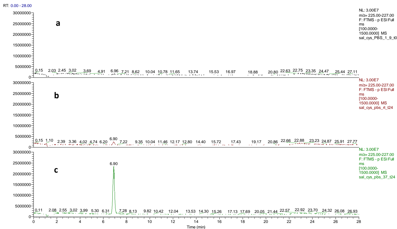
Figure S1: ESI negative mode extracted ion chromatograms (m/z 225-227) of saligenin-cysteine mixture in PBS buffer (a) directly after mixing saligenin with cysteine (b) after 24 h of incubation at room temperature (c) after 24 h of incubation at 37°C.
