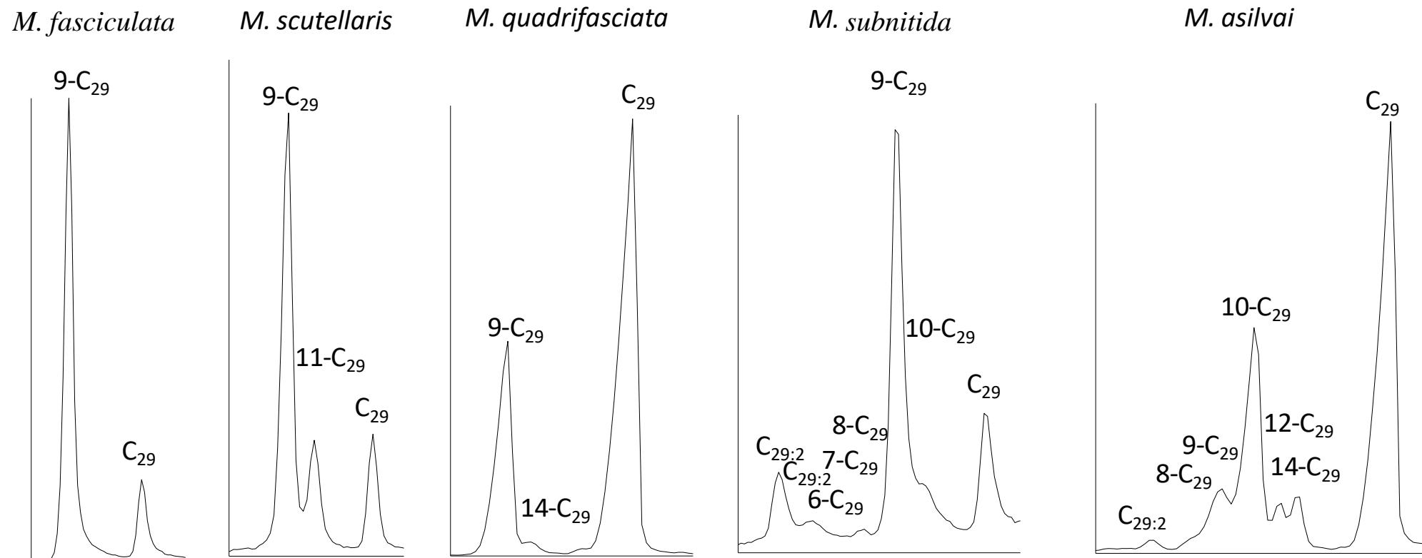
Fig. S7. A section of the TIC's for five species of *Melipona* and the corresponding C<sub>29</sub> alkene isomers revealed by the DMDS reactions.
